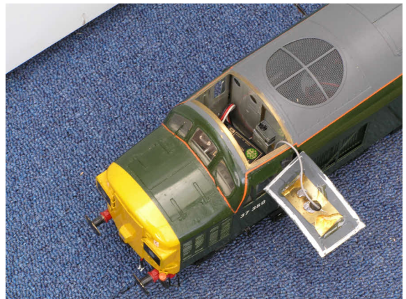
40MHz FM Aerial Set-up for a B.R. Class 37 Diesel Loco In this case the roof is a fabricated clip-in plasticard panel pre-formed between two strips of metal with a heat gun. The roof enables access to the receiver in the cab, as well as providing an isolated area for the brass pickup plate to which the aerial is connected. The loco has a nickel silver body, and brass chassis with whitmetal castings.
