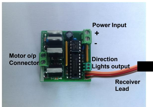
The '+' power input terminal is marked with a red spot. **'Tin' all multi-stranded wire connections with solder, before clamping in the terminals.** Do not over-tighten the terminals. Note that the clamps in the screw terminals rise when tightened, so put wires above the clamps, not below.
